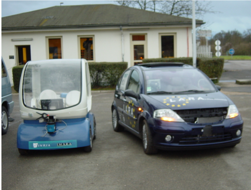
Figure 2.1: A CyCab (left) and a Citroën C3 (right), the two main platforms used at Imara. Reproduced with permission from Imara, courtesy of Laurent BOURAOUI.
